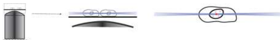
Figure: Schematic of light sheet illumination for single-molecule imaging. Only fluorophores in the light sheet are excited.
